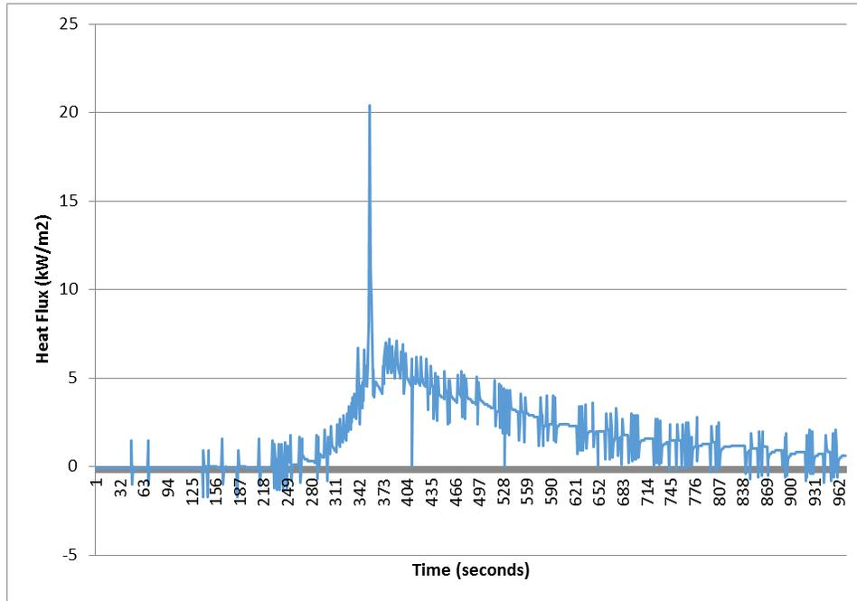
Figure 2. Heat flux profile from the sensor in the short box.
