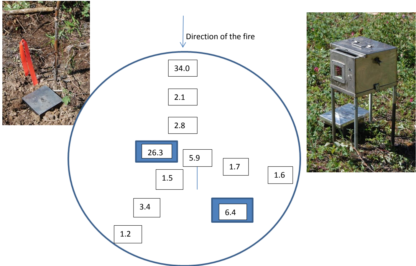
Figure 3. Heat flux values (kW/m 2 ) inside the 10 m opening. The fire entered the opening at the top.
