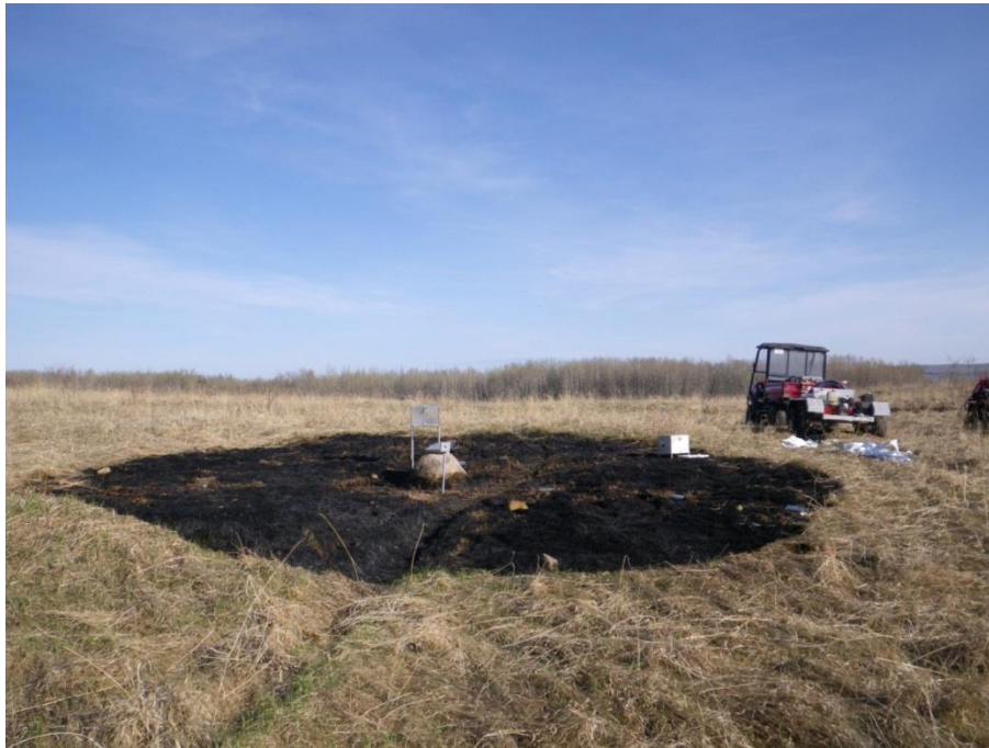
Figure 1. The 10 m survival opening instrumented with flat sensors, 2 cameras and a cube sensor.
