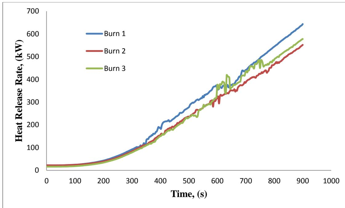
**Figure 5:** Heat release rate of three experimental burns with a feather moss fuel bed treated with water at coverage level 4.
