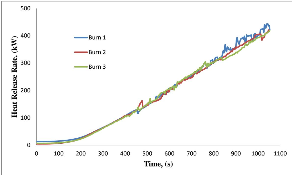
**Figure 9:** Heat release rate of three experimental burns with a feather moss fuel bed treated with Gel Product C at coverage level 4.
