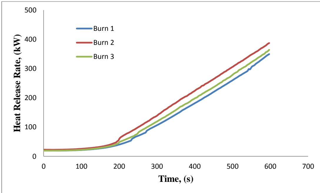
**Figure 4:** Heat release rate of three experimental burns with a feather moss fuel bed and zero coverage level.
