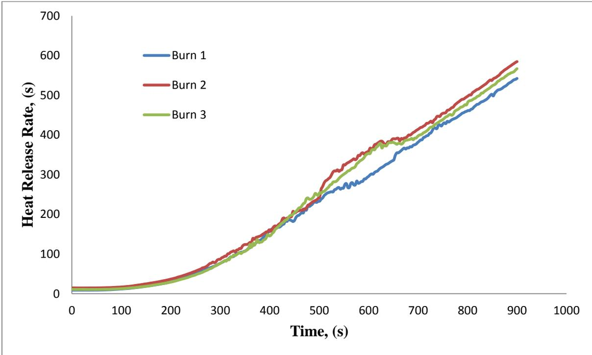
**Figure 7:** Heat release rate of three experimental burns with a feather moss fuel bed treated with Gel Product A at coverage level 4.
