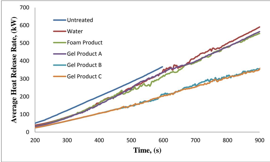
**Figure 12:** Comparison of average heat release rates between water, Foam Product, Gel Product A, Gel Product B, and Gel Product C.
