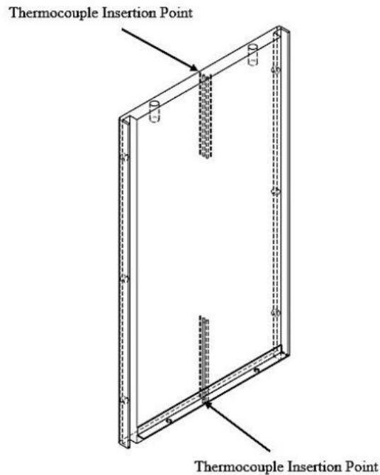
**Figure 3:** Representation of Thermal Canister Walls [1]
