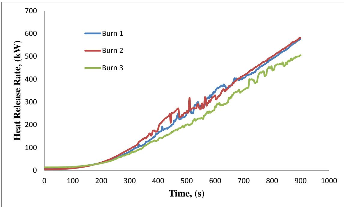
**Figure 6:** Heat release rate of three experimental burns with a feather moss fuel bed treated with the Foam Product at coverage level 4.
