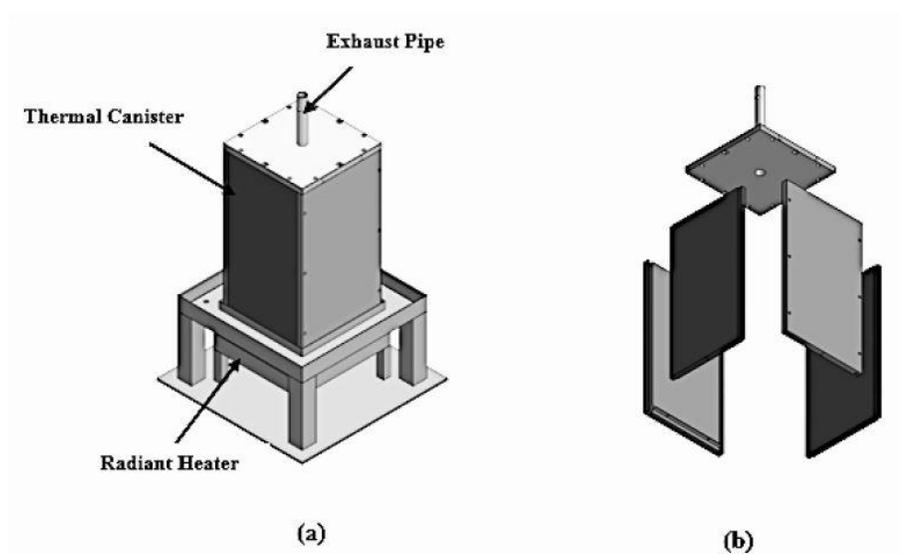
**Figure 2:** a) Thermal Canister Assembled, b) Exploded view of Thermal Canister [1]
