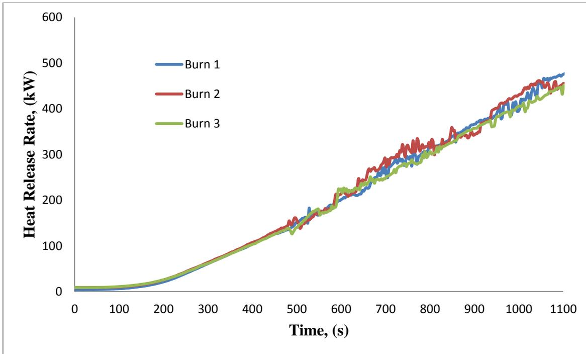
**Figure 8:** Heat release rate of three experimental burns with a feather moss fuel bed treated with Gel Product B at coverage level 4.
