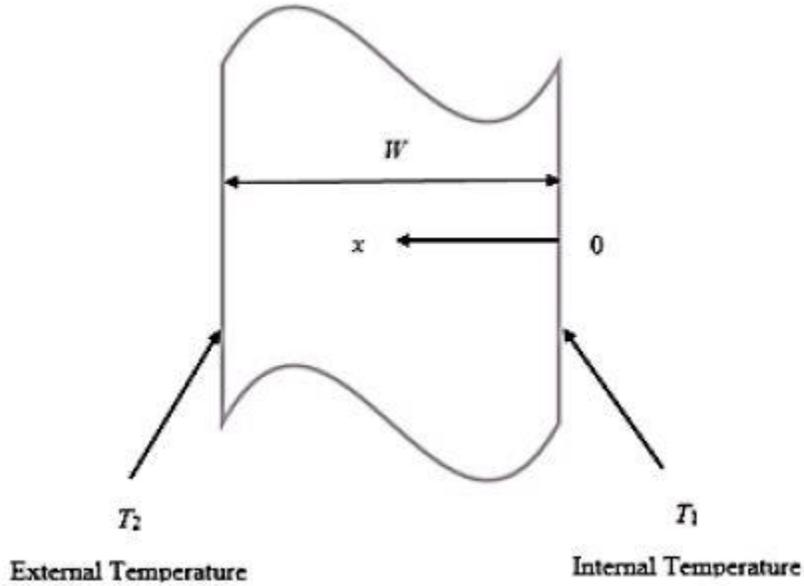
**Figure 1:** Representation of the thermal canister wall showing the boundary conditions [1]
