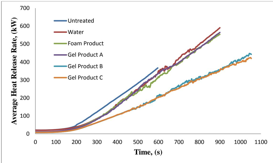
**Figure 10:** Comparison of average heat release rates between different fuel treatments
