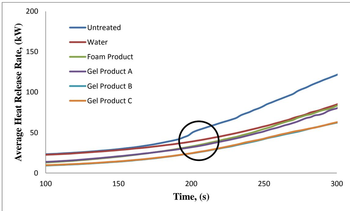
**Figure 11:** Onset of combustion process in the untreated fuel in comparison to the treated fuels
