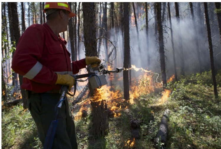
Figure 5. The Dackermin Torch in use on an experimental burn at the CBCFS project site.
