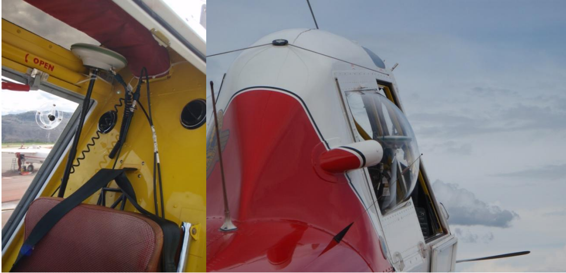
Figure 2: GPS antenna securely attached inside the aircraft.
