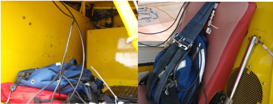
Figure 3: GPS receiver mounted in baggage compartment (left) and on rear seat (right).
