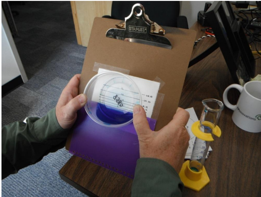
Figure 1. Template calibration with measured amount of water for GPC7 (coloured water used for visibility)
