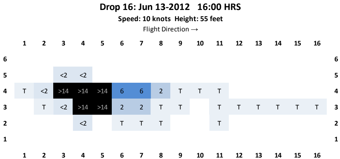
Figure 4. Presentation of direct measurement point data (in GPC) from drop tests.
