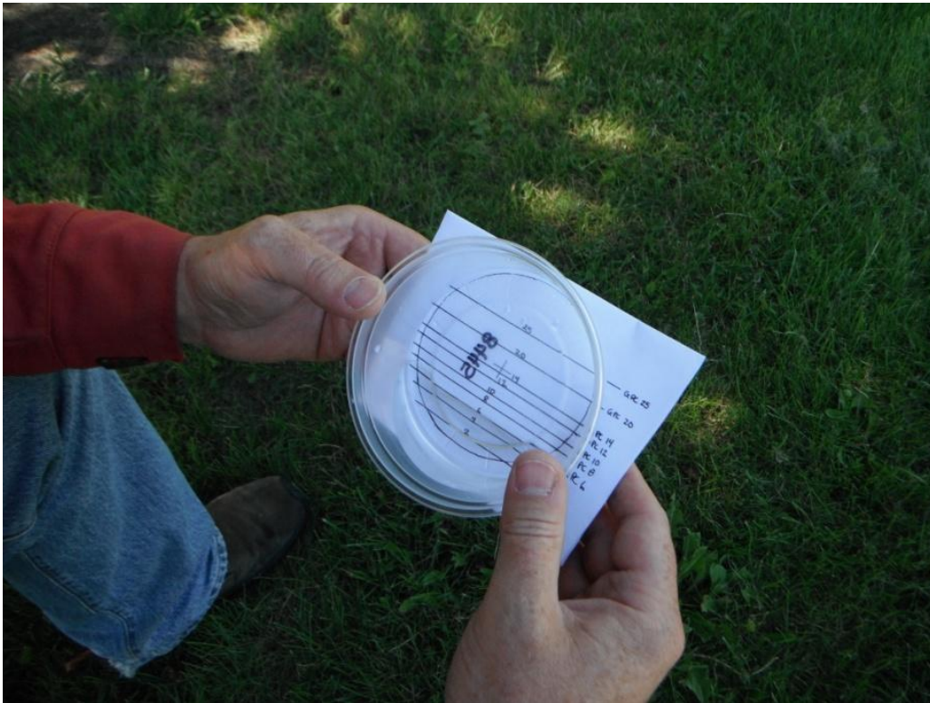
Figure 3. Using the template to directly measure coverage level.
