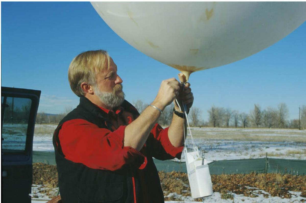
Figure 2. Radiosonde being prepared for release. Courtesy of the Digital Image Library, UCAR.
