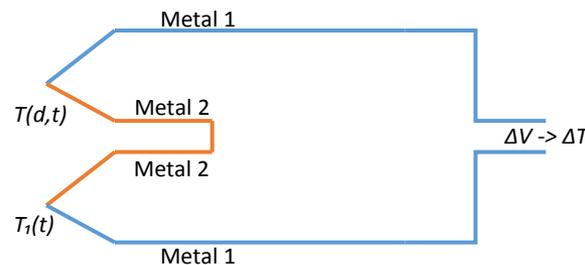
Fig 2: Thermocouple Circuit to obtain  $\Delta T$
