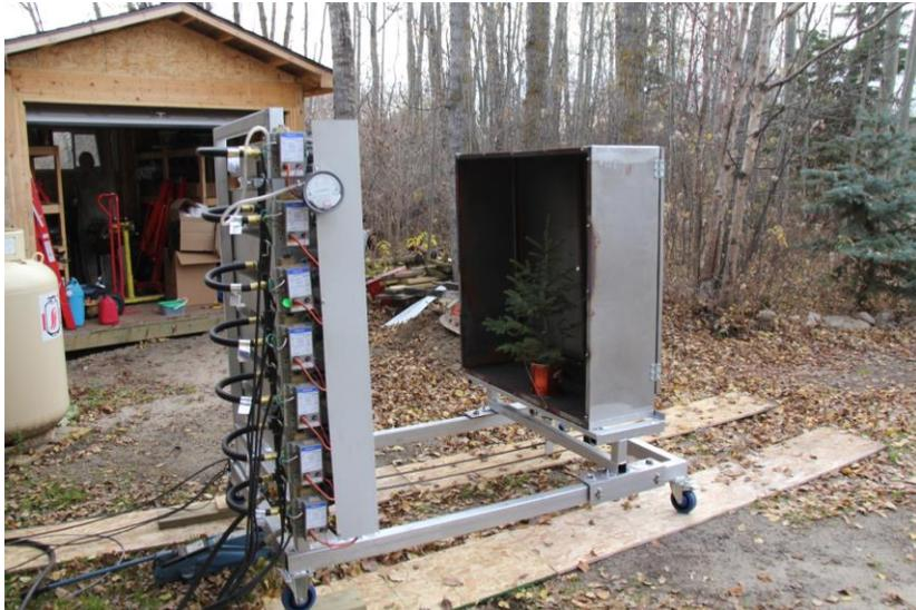
Figure 1. The radiant panel we plan to use for sensor calibration.
