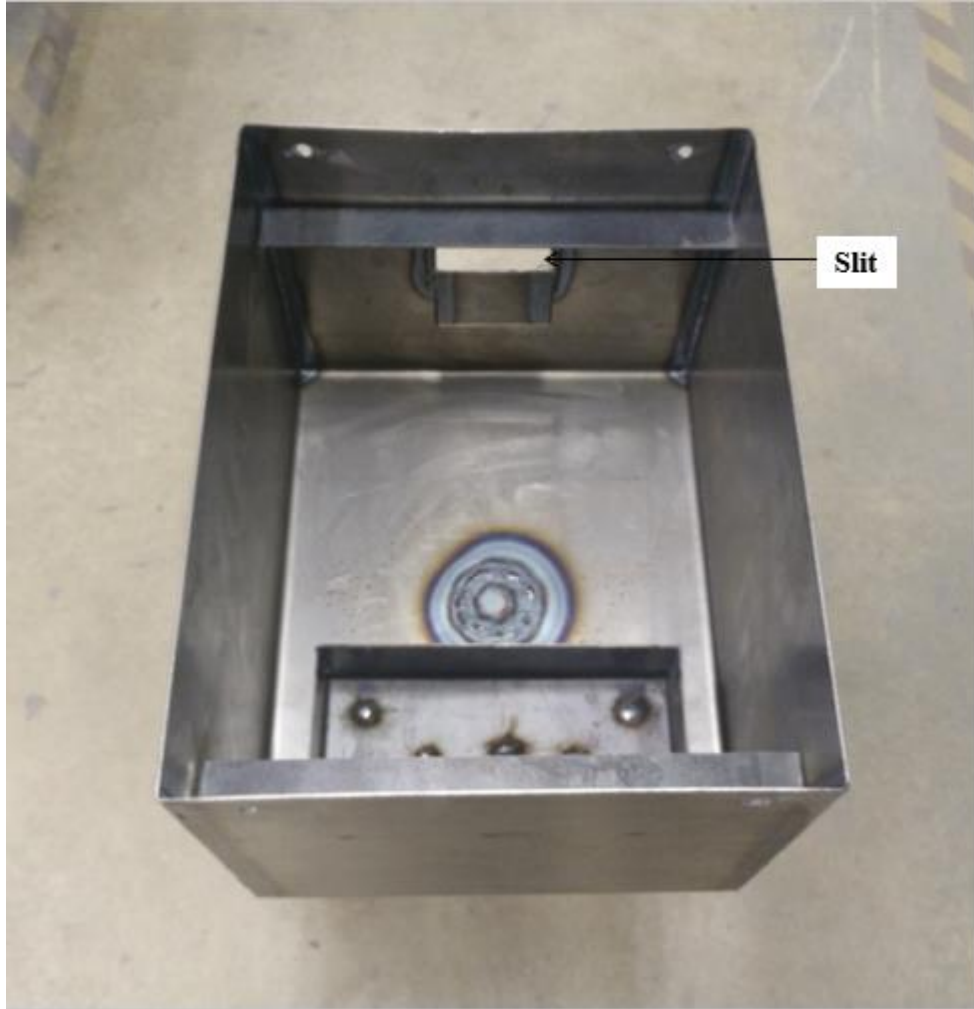
Figure 5: Slit for routing of thermocouples in the Main Box
