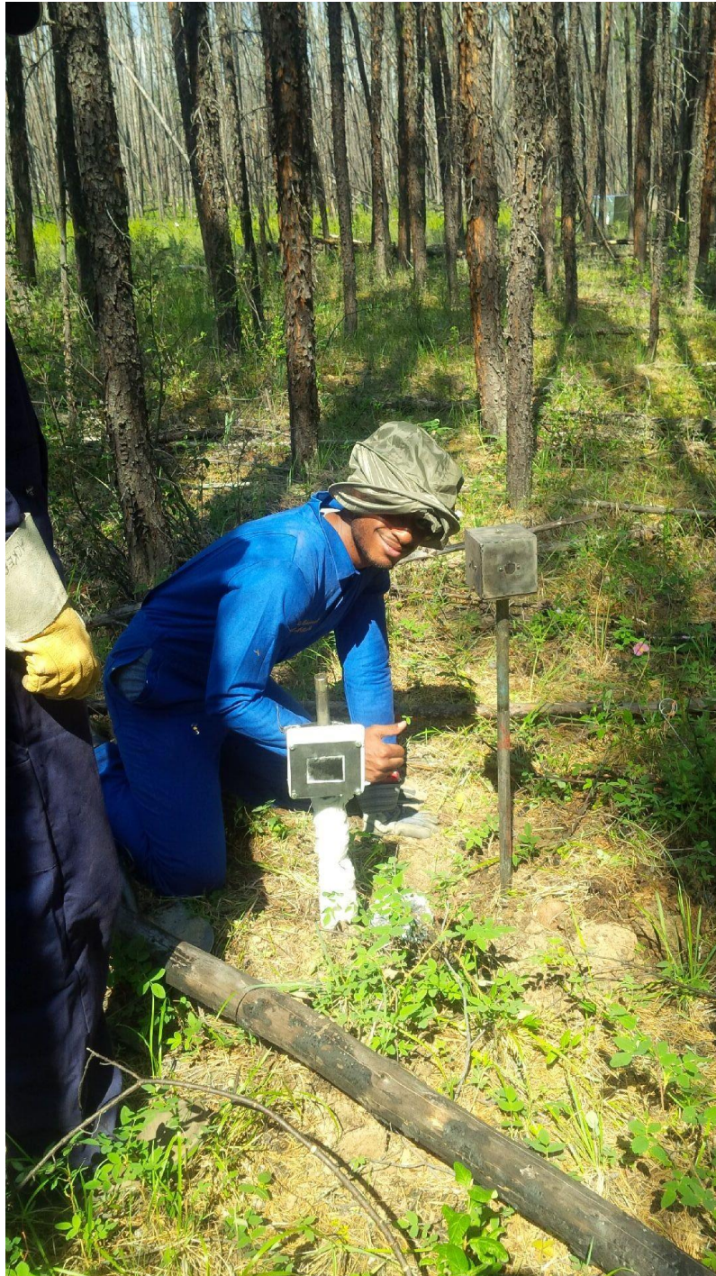
Figure 1. Heat flux sensor testing in the Northwest Territories (2014).
