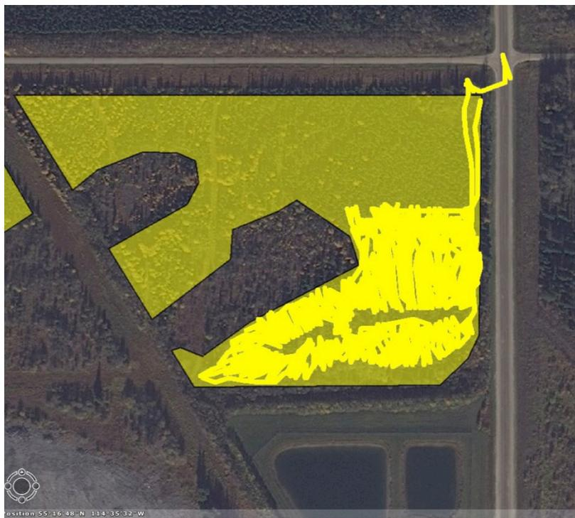
**Figure 3. GPS track (bright yellow) of the piling operation for the D7 dozer on February 18, 2014.**
