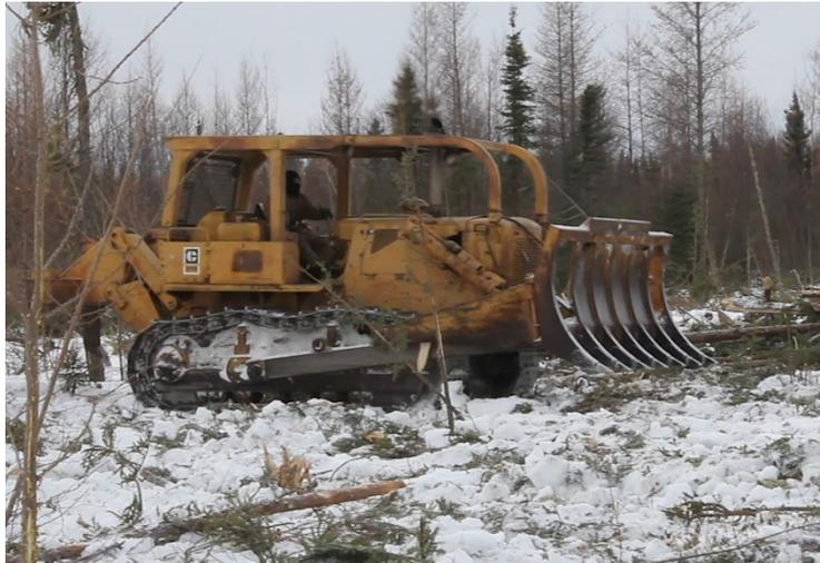
Figure 1. The Caterpillar D7G dozer with a brush rake attachment.
