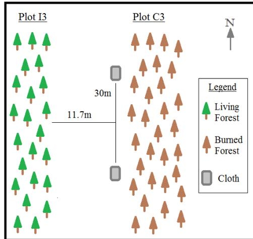
Figure 1. Diagram of Plot I3 that shows two sheets: one positioned north and one positioned south relative to each other. The sheets were positioned downwind of the plot to maximize firebrand collection. Diagram is not to scale.
