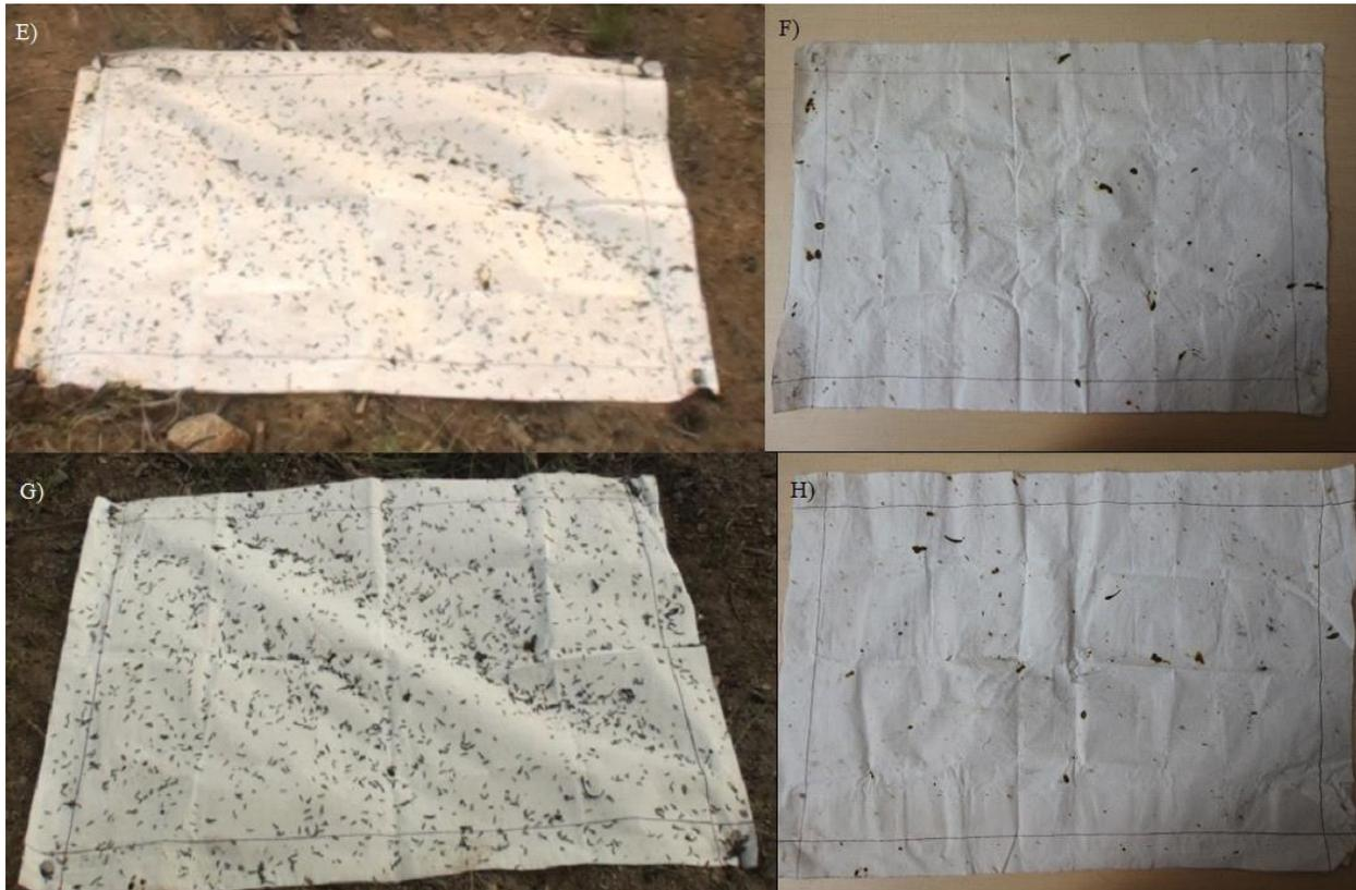
**Figure 4.** The images on the left are from the video showing firebrands at a high-density point during the fire (images E and G). The images on the right show the burn marks on the sheets (images F and H). Images E and F are from the Triangle Plot sheet ID “1E” and images G and H are from the Triangle Plot sheet ID “1W”.
