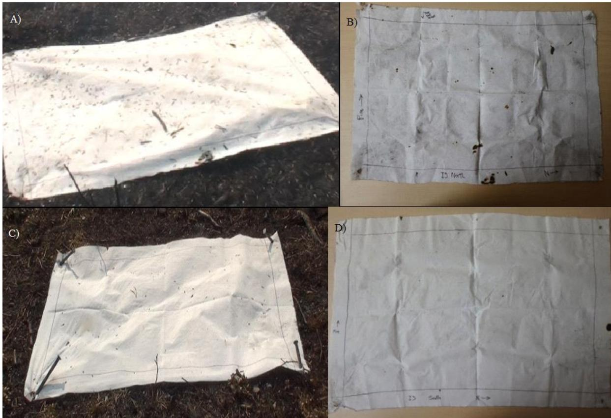
**Figure 3. The images on the left are from the video with firebrands at a high-density point during the fire (image A and C). The images on the right show the burn marks on the sheets (images B and D). Image A and B are from Plot I3 sheet ID “2N” and images C and D are from Plot I3 sheet ID “1S”.**
