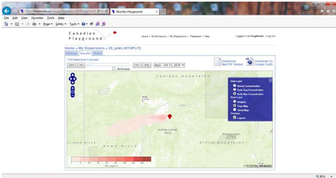
Figure 3. Smoke dispersal scenario for the burning of 30 windrows on October 13, 2016.
