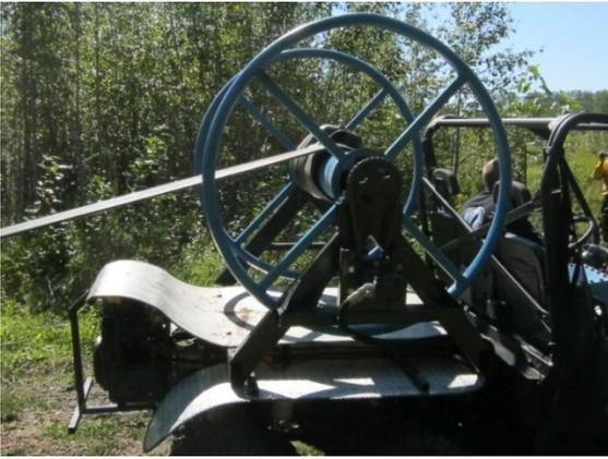
**Figure 3. The reel system on unit two spooling the 4 inch hose**
