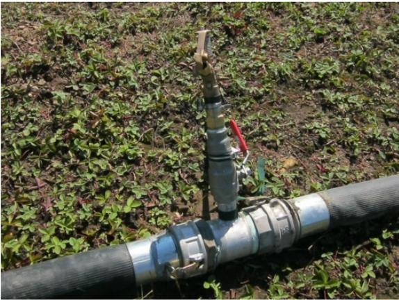
Figure 2. Cam lock fitting and 1½ inch fitting for sprinklers
