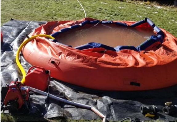
Figure 5(a). WICK 375 connected to a 9,463-L. (2,500-gallon) bladder.
