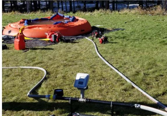
Figure 5(b). Flow meter and pressure gauge 30-m. (100-ft.) from pump.
