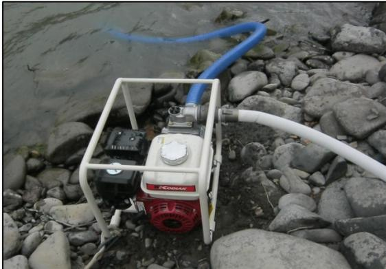
Figure 3. Honda WH20XTC pressure pump.
