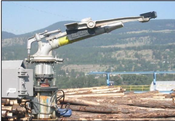
Figure 1. The Big Gun SR100 sprinkler with a TWIG wireless decoder box.
