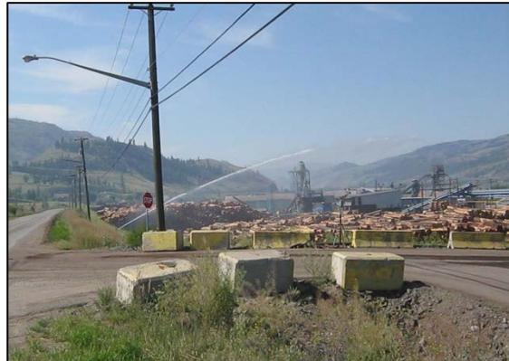
Figure 4. The Big Gun sprinkler in operation at the Tolko millyard at the Heffley Creek saw mill. Spray distance is approximately 30-61 m (100–120 ft.).
