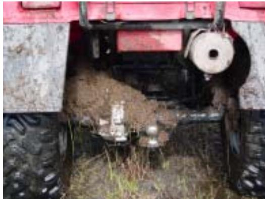
Figure 5. Steam observed on the exhaust system of an ATV. Note that the rear of the muffler is already dry.
