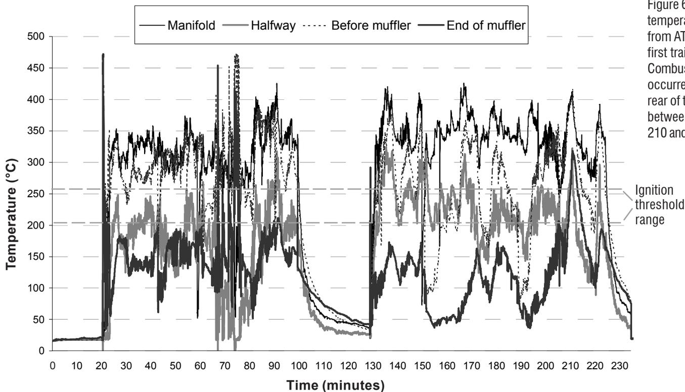
Figure 6. The time-temperature traces from ATV 3 for the first trail ride. Combustion occurred on the rear of the muffler between minutes 210 and 220.
