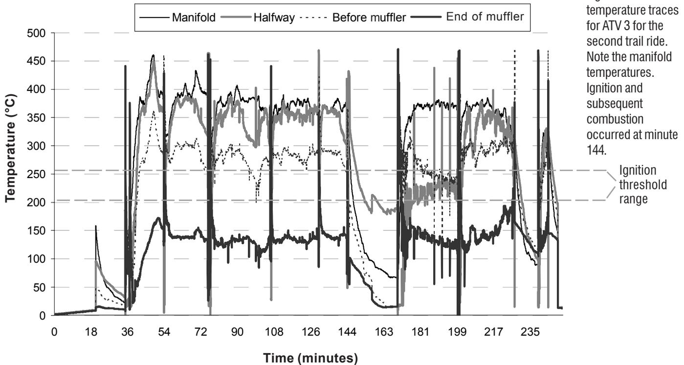
Figure 10. Time-temperature traces for ATV 3 for the second trail ride. Note the manifold temperatures. Ignition and subsequent combustion occurred at minute 144.
