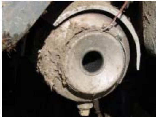
Figure 9. Two smouldering points and scorched areas on the muffler from which debris had fallen to the ground. Some smoke is visible as well.
