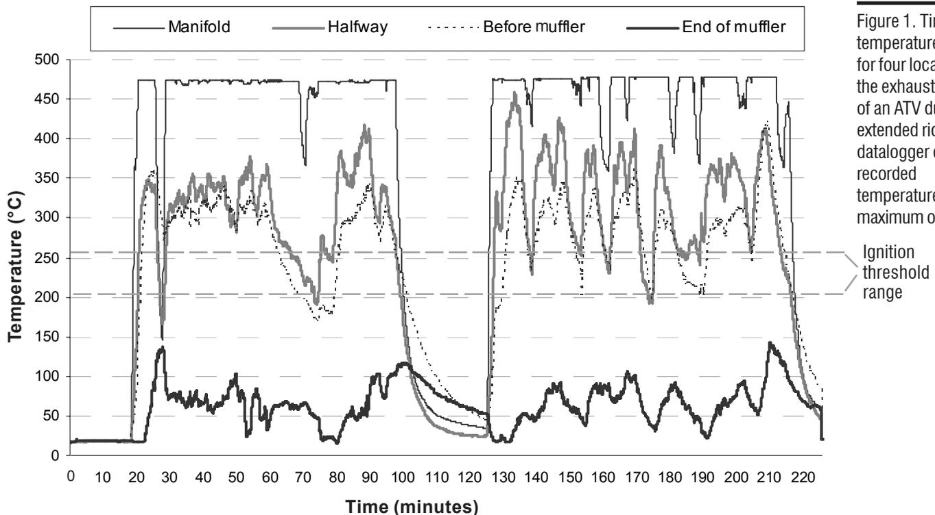
Figure 1. Time-temperature traces for four locations on the exhaust system of an ATV during an extended ride. The datalogger only recorded temperatures to a maximum of 475°C.
