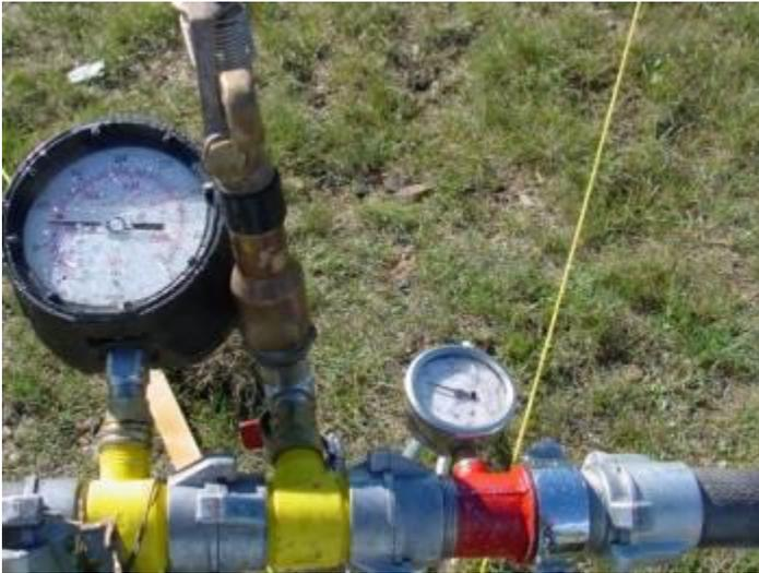
Figure 7. Pressure gauges placed directly before and after the sprinkler head to determine if there was any drop in pressure.
