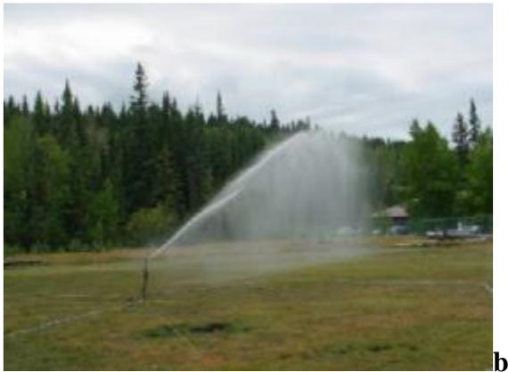
**Figure 17 a-b.** The ‘snow-like’ appearance created during foam testing. The mist curtain below the main spray results from the foam.
