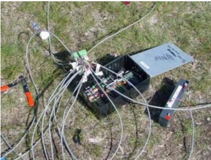
Figure 9. Data loggers downloaded temperature and RH data every second from the 17 sensors locations.
