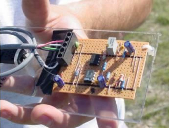
Figure 10. The circuit board and RH sensor used in the sprinkler trials.
