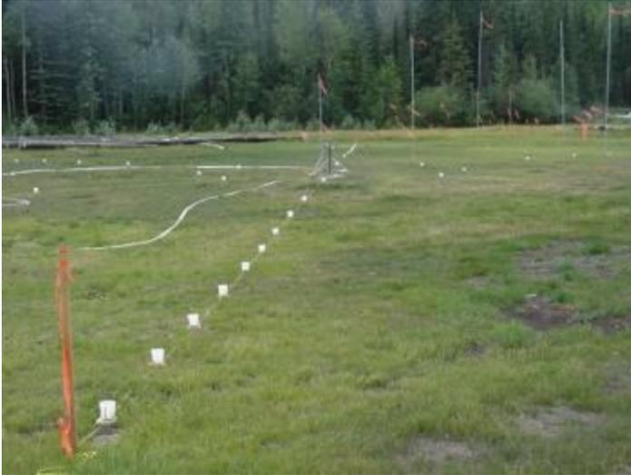
Figure 12. Volume cups were spaced for equal area on eight quadrants of the compass to collect water for determining the distribution (footprint) pattern of water over the area.
