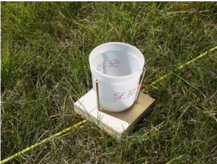
Figure 13. Cups are 9 cm high with a 9 cm diameter opening. A piece of green turf was placed in bottom of cup to prevent water from splashing out. Each cup was weighed dry and again with the water to determined volume collected. Each cup is marked and placed at a specific point on the quadrant.
