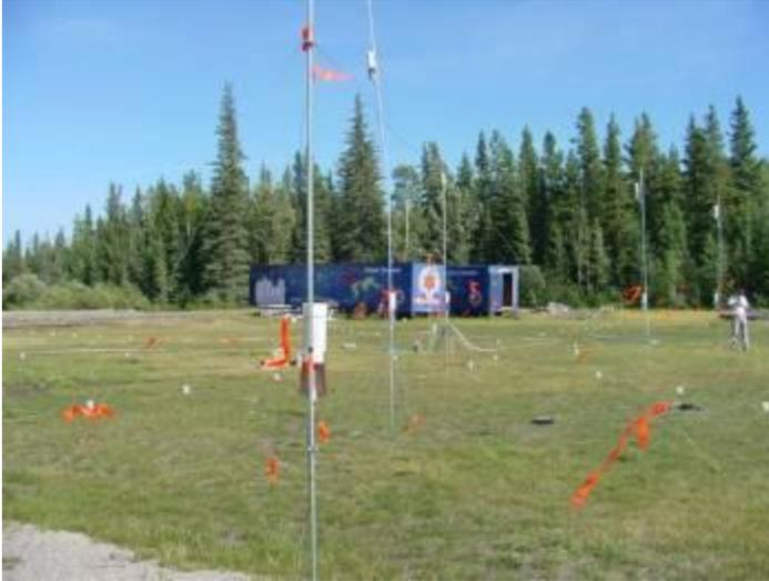
Figure 8. Relative humidity and temperature sensors in protective cases measuring changes in RH and Temperature above and below the water from the sprinkler head.
