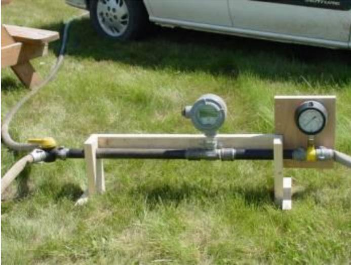
Figure 4. Flow meter and pressure gauge on stand located 10 feet from the Mark III pump.
